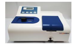
A spectrophotometer is an instrument that measures the amount of light absorbed by a sample. Spectrophotometer techniques are mostly used to measure the concentration of solutes in solution by measuring the amount of the light that is absorbed by the solution in a cuvette placed in the spectrophotometer.
