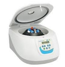
• It is a device that uses centrifugal force to subject a specimen to a specified constant force, for example to separate various components of a fluid.
