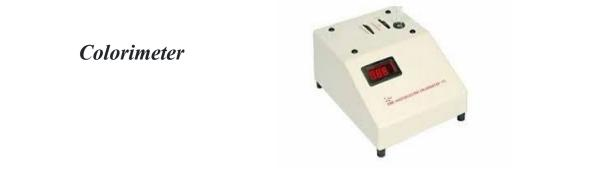
• A **colorimeter** is a tool that detects how different liquids absorb specific colors of light. It measures how much light gets absorbed and how much passes through the liquid. Basically, when you shine a specific color of light through a colored liquid, the colorimeter tells you how much of that light gets absorbed.
